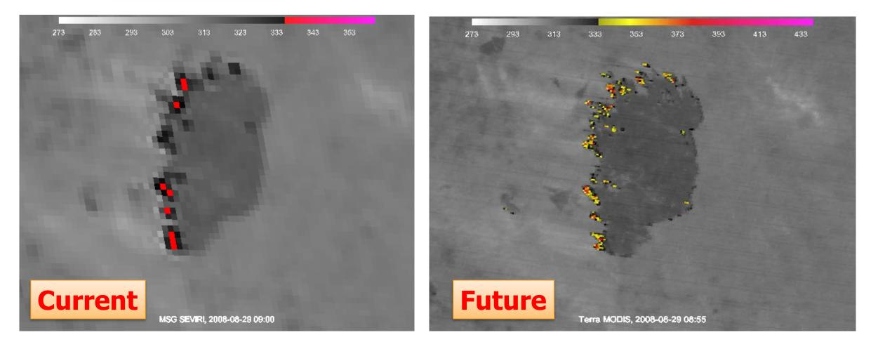
Bushfire line in Botswana as seen in imagery from current Meteosat (left panel) compared to future MTG imagery simulated by proxy data (right panel). MTG imagery will enable more precise detection of fire location and better fire intensity estimates.
