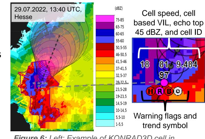
Figure 6: Left: Example of KONRAD3D cell in meteorological workstation NinJo with contour polygon and uncertainty ellipses around forecast centroids. Right: Zoom on 2D-centroid.
