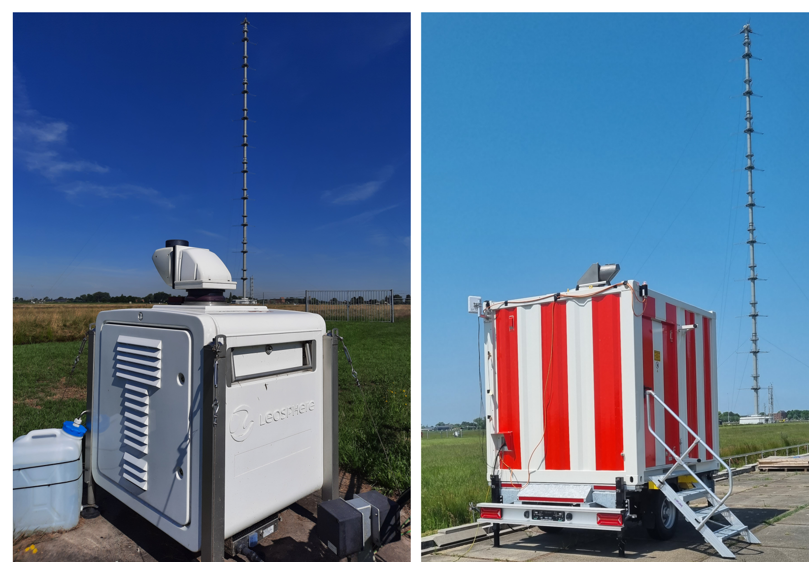
Figure 5: Long-range scanning Doppler lidars at Cabauw: (left) Windcube200S, (right) Skiron3D. In the back the 213-m tall tower of Cabauw.
