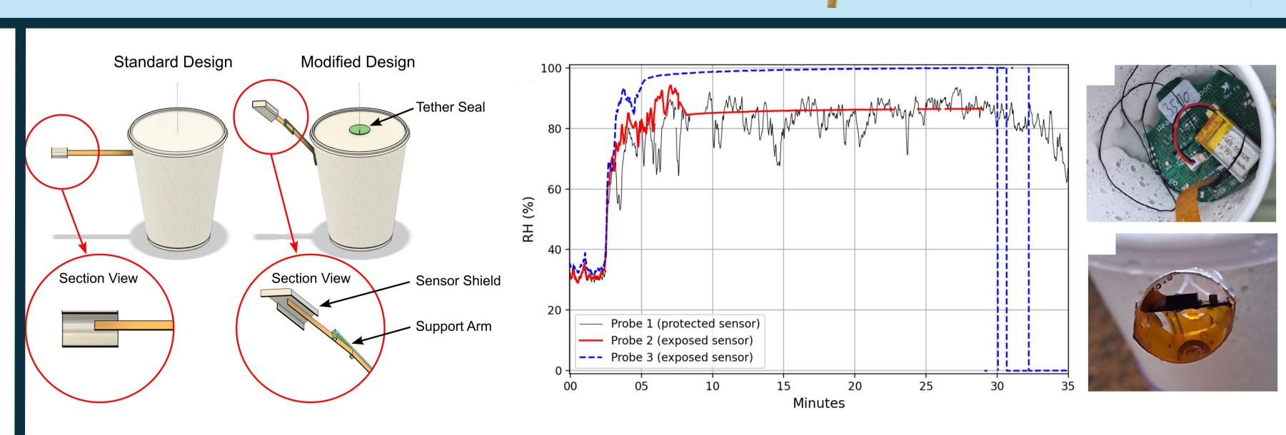
INSTRUMENT MODIFICATIONS: Modifications were made to protect the Windsonds' temperature and relative humidity sensors from precipitation<sup>1</sup>. Common sensor failure modes from water ingress: suppressed relative humidity (RH) variability (probes 2 & 3), software re-initializations and power failure (probe 2), erroneous RH saturation and folding (probe 3).
