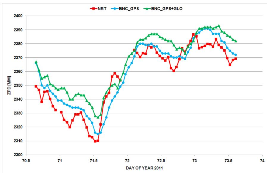
**Figure 7:** ZPD estimates from BNC26 for station KARL using clock corrections CLK10 (GPS) and CLK11 (GPS+GLO)
