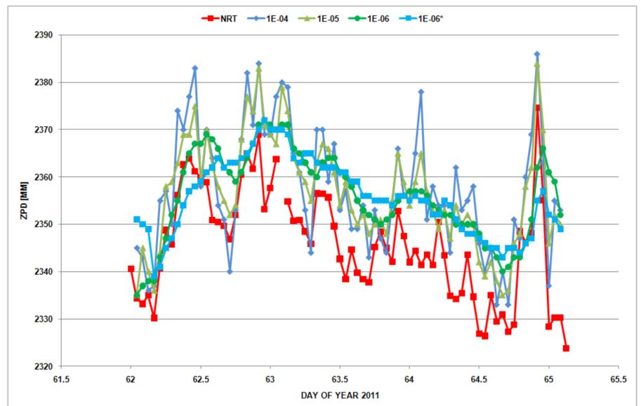
**Figure 6:** ZPD estimates from BNC26 for station KARL using clock corrections CLK11 (GPS+GLO) and different settings for tropo white noise, compared to NRT results. Smoothing effect when constraining with 1e-06 (or less) \* solution without fixing the coordinates
