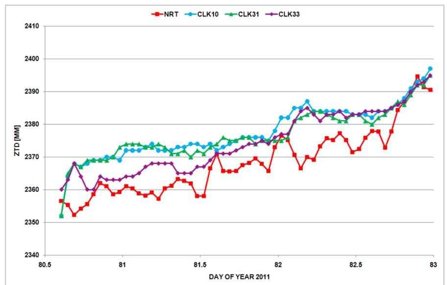
**Figure 8:** ZPD estimates from BNC26 for station KARL using clock corrections CLK10 (individual contribution from BKG), CLK31 (combined solution from IGS-RT PP) and CLK33 (combined solution with BNC)
