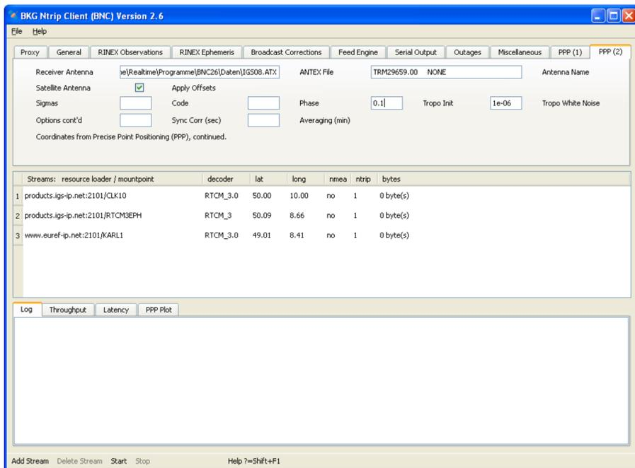
**Figure 5:** Menu of BNC for PPP application; choosing of appropriate values for Tropo initialisation and white noise combined with fixing coordinates (see Figure 1) allows individual estimation of zenith total delay parameters.
