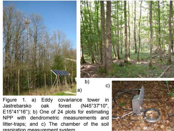
Figure 1. a) Eddy covariance tower in Jastrebarsko oak forest (N45°37'10", E15°41'16"); b) One of 24 plots for estimating NPP with dendrometric measurements and litter-traps; and c) The chamber of the soil respiration measurement system.
