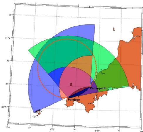
**Figure 1:** HF radar coverage map for Wave Hub site. Each station covers a 120 degree sector and surface velocity measurements are available for full range of sector while directional wave measurements can be obtained from inner region.
