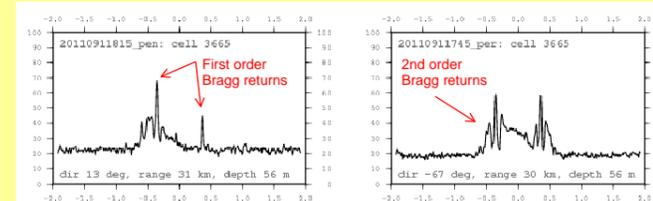
**Figure 5:** Frequency spectra from detected signal (beam formed) at Pendeen and Perranporth. Strong peaks from Bragg scattering are easily identified (+/-) and deviations from symmetry indicate additional radial current. Returns from two stations permit the resolution of current direction.
