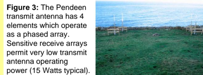
**Figure 3:** The Pendeen transmit antenna has 4 elements which operate as a phased array. Sensitive receive arrays permit very low transmit antenna operating power (15 Watts typical).
