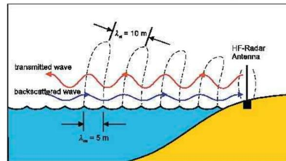
**Figure 4:** Bragg scattering of transmitted HF radar signal results in strong return at Doppler frequency related to phase speed of gravity waves with half the  $\lambda$  of the radar waves. (© Klaus-Werner Gurgel, University of Hamburg, Germany)
