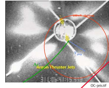
Luminosity disappears 15 s after separation, i.e., after evacuation time, so the light is excited Argon.
