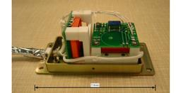
Fluxgate magnetometer sensor
