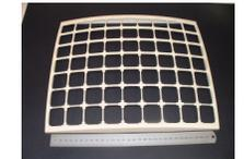
Example frame constructed at Leicester University for holding individual MCP plates
