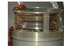
Prototype of the top-hat analyser suitable for implementation as the PAS
