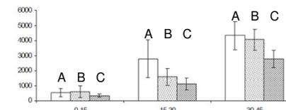
Figure 2: Average maximum soil resistance (Y-axis; kPa) within each block (A, B, C) for three soil depths (X-axis; cm); with standard deviations.
