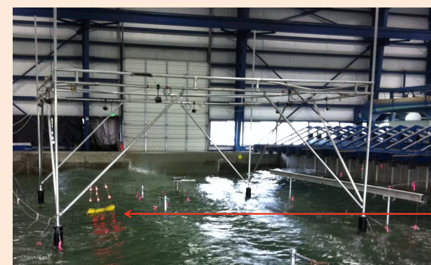
Observations included PhaseSpace© motion capture system for WEC performance analysis and stereo video for 3D water surface reconstruction.
