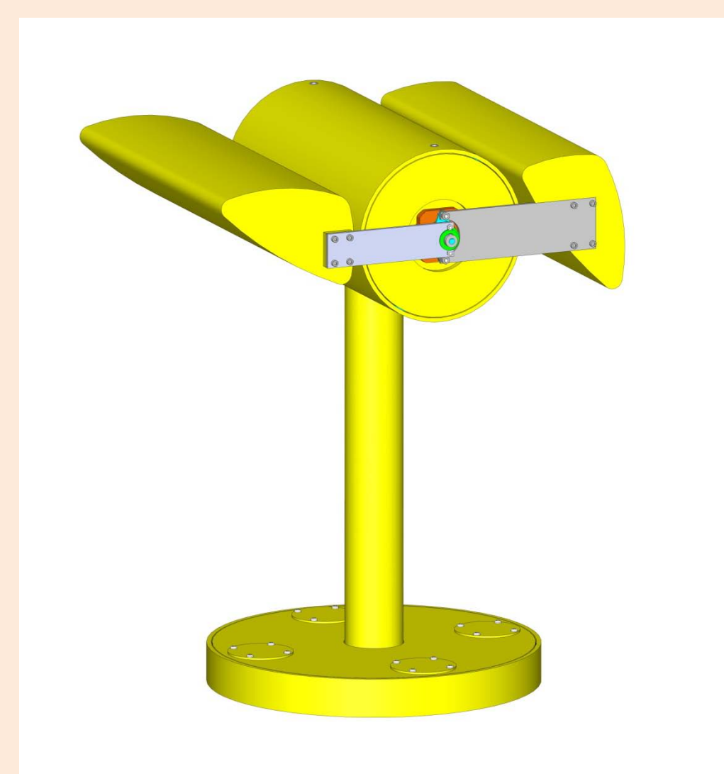
Five 1:33 scale “Manta” Wave Energy Converters (CPT) were used in the experiments
