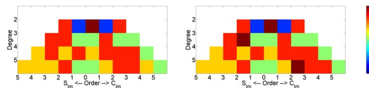
Fig. 2: Number of reproduced digits without leading zeros w.r.t. EGM2008 based on data collected over one month (left) and twelve months (right).
