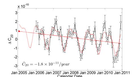
Fig. 3: Monthly values of  $\Delta C_{20}$  w.r.t. EIGEN-5S (black circles) with standard deviations (black error bars). The variation has been fit by a regression line (straight red line) together with annual and semiannual sinusoids (curved red line). The coefficient has been extrapolated (red triangle) along the extrapolated regression line (dashed red line) to January 1, 2005.
