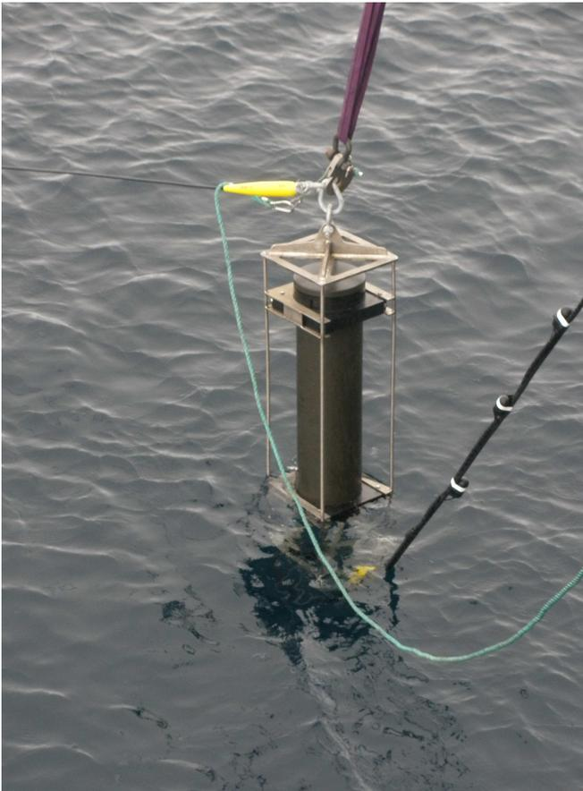
Bjørge Naxys system is integrated with the tomography instruments @ 350 m in 2580 m water depth.
