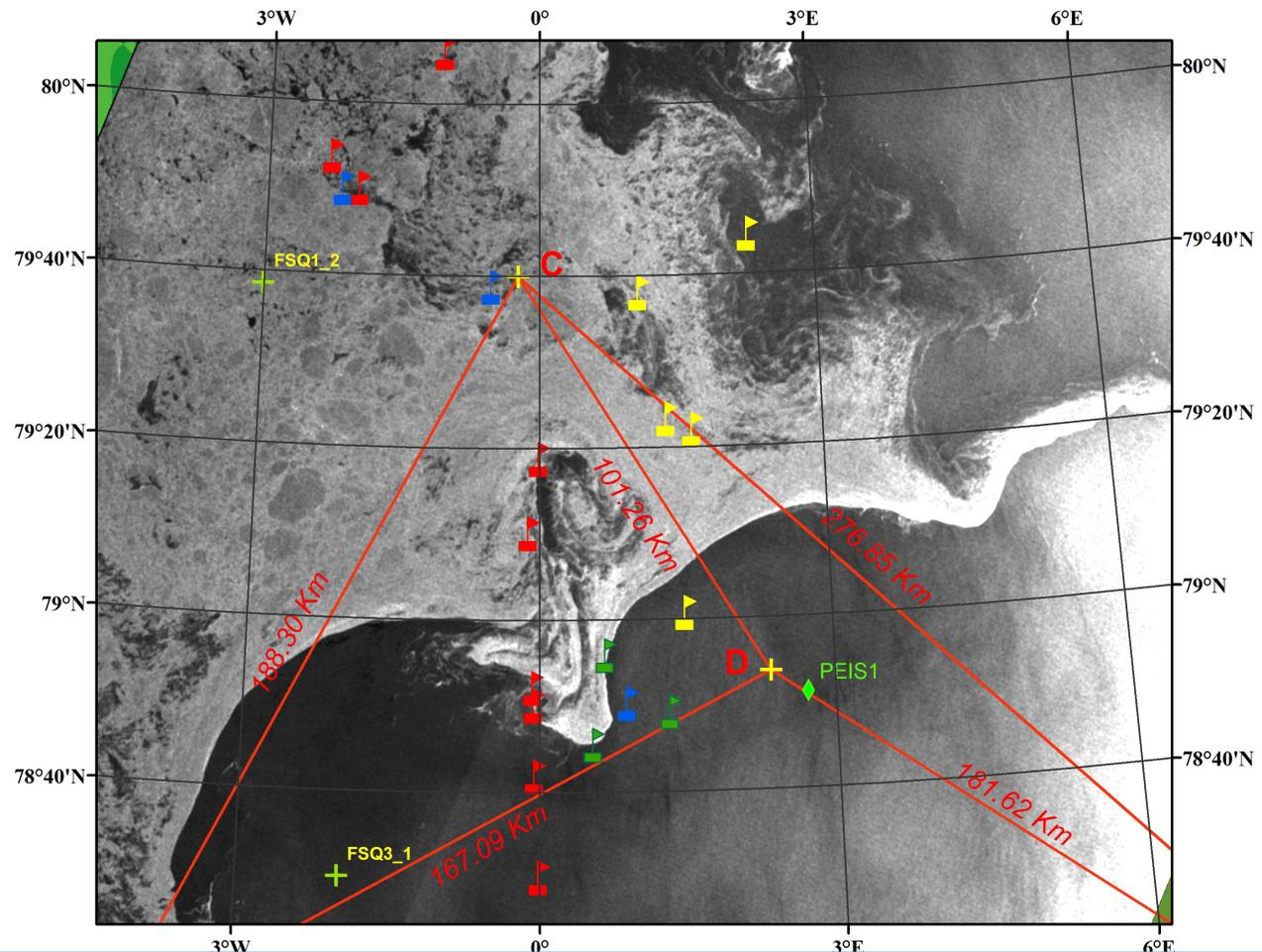
Red/green flags – hydrophone at 305 m, Yellow flags hydrophone at 122 m, Blue flags AXBTs C&D is tomographic moorings, FSQ moorings are RAFOS sources, and PEIS is inverted echo sounders. This is work carried out with FFI in Horten.
