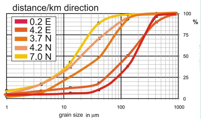
Fig.3: Grain size distributions of the mineral components of the pure fly ash (red, distance 0.2km) and of fly ash enriched forest floor horizons with increasing distance to the main emission source [C].
