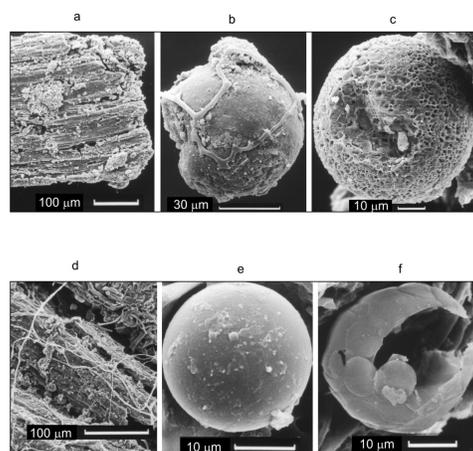
Fig. 2: Scanning electron micrographs of the pure fly ash (a-c) and of a fly ash enriched forest floor horizon (d-f). a: lignite rest; b,c and e,f: mineral fly ash particle; d: organic structure. [C]
