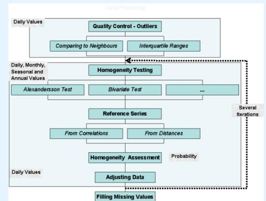
Scheme of usual data processing during data quality control and homogenization (preparing data for time series analysis)
