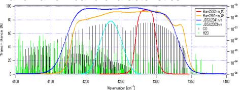
Total sensitivity test by using CO gas cell with combination of 2.3 micron detector and BPF installed on the TANSO-FTS breadboard model.
