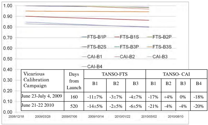
Band1 FTS and CAI degradation may have occurred just after launch or may be due to a pre-launch calibration error.
