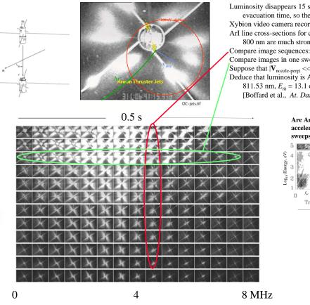
Luminosity disappears 15 s after separation , i.e., after evacuation time, so the light is excited Argon.
