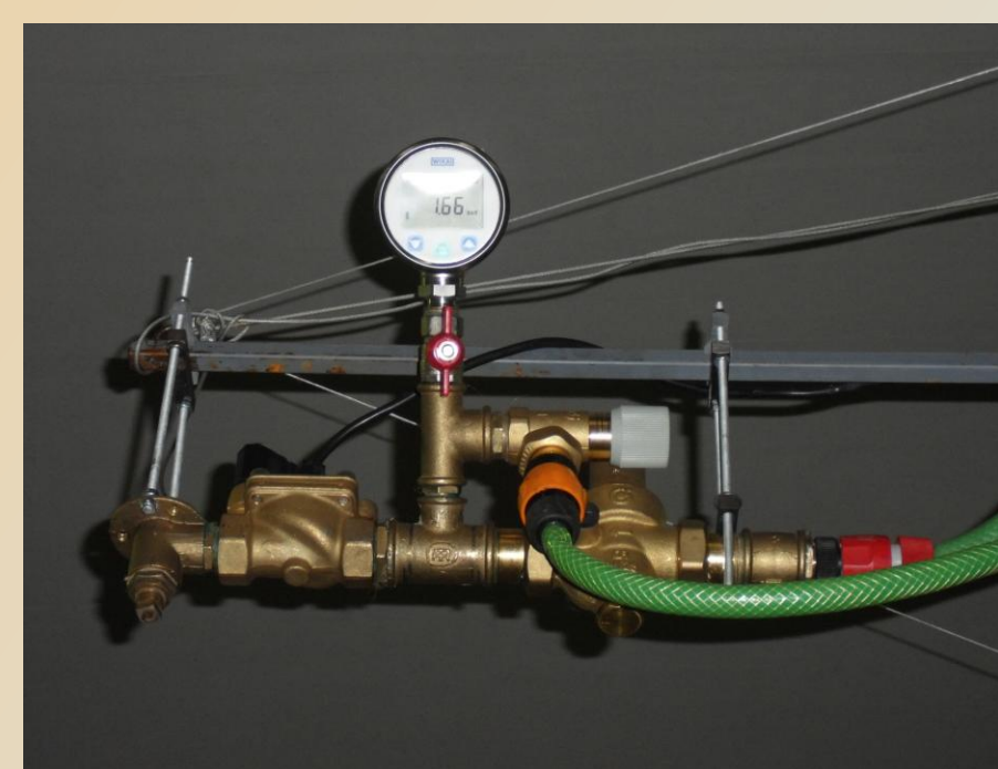
Figure 4 – Flow control system.
