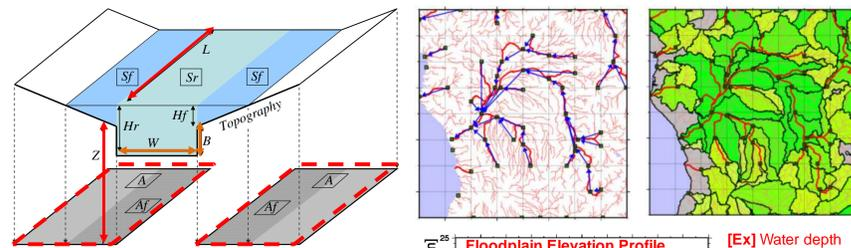
**Red Parameters:** from 90-m resolution HydroSHEDS with DEM modification [Yamazaki et al. (submitted to JH)]
