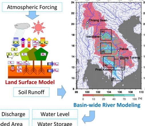
Instead, we applied a continental-scale distributed hydrodynamics model, CaMa-Flood, for the entire Mekong River in order to simulate the seasonal cycle of flooding extent without using the upstream boundary inflows to the model.
