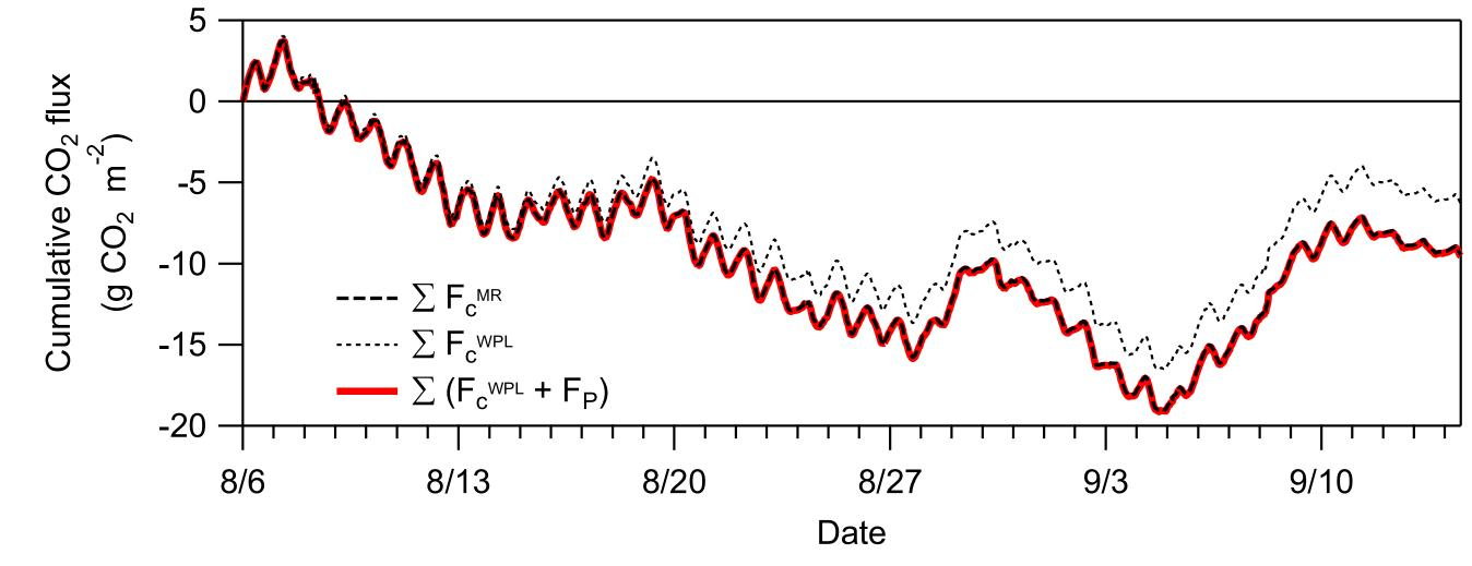
This study is the first to actually confirm by experiment that  $F_c^{MR}$  and  $F_c^{WPL} + F_P$  are identical. To reduce uncertainties in calculations, we recommend using the mixing ratio for calculation of  $CO_2$  fluxes when using the new type closed-path infrared gas analyzer.
