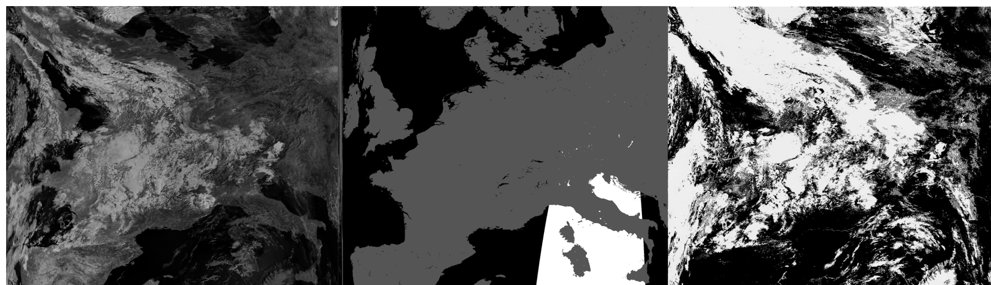
Fig.1: APOLLO algorithm applied for one 2048x2048 km² MetOp frame over Europe on 01.09.2008. Left frame corresponds to the reflectances from AVHRR/MetOp Channel 3 without cloud correction. Middle frame represents land-sea mask and sun glint mask derived from APOLLO. Right slide shows cloud mask with 1 km² resolution, which later is used in SYNAER/MetOp retrieval in order to eliminate and discern between cloudy pixels and pixels with aerosol load.
