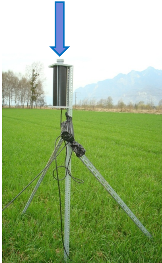
Air-O-Cell pollen sampler (vertically oriented orifice) air throughput 18 l/min
