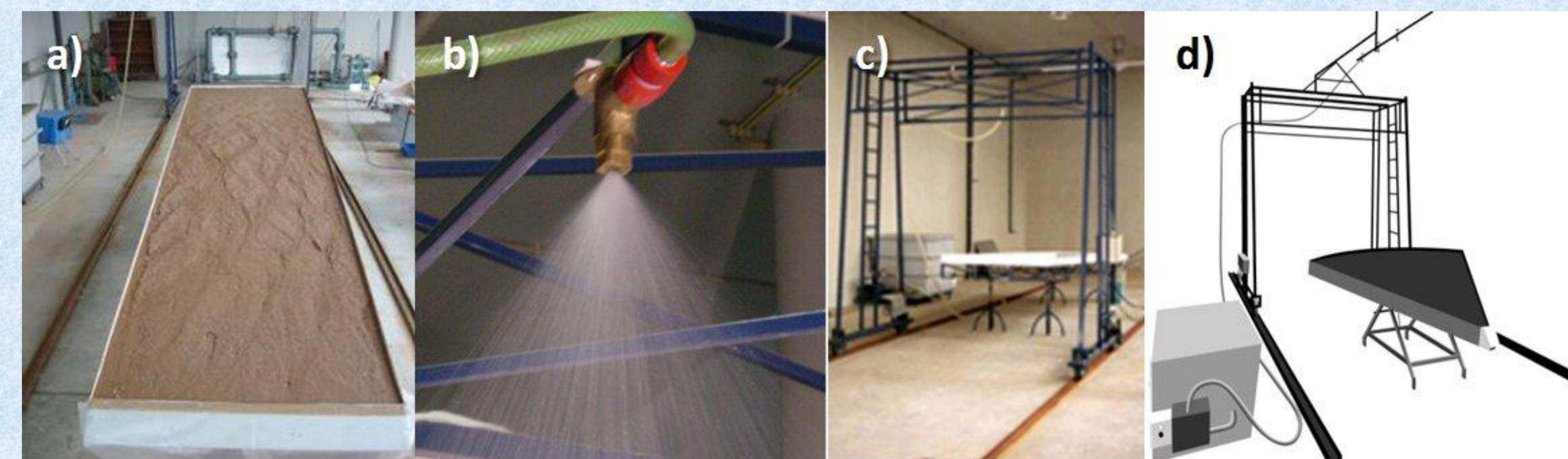
Fig. 1 – Photographs of a) flume, b) full-cone nozzle spray, c) rainfall simulator installed on a structure that is electrically driven along rails and d) sketch of the laboratory set-up with a converging flume surface.
