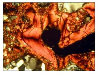
**3Btg** (100X-XPL): thick laminated clay coating with sharp extinction band
