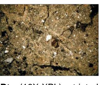
Btg (16X-XPL): striated b-fabric due to oriented clay domains.
