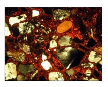
3Btg (40X-XPL): high illuvial clay degree of infillings.
