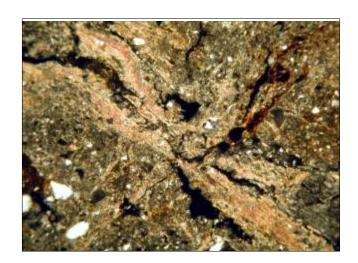
Btg (40X-XPL): stress deformed clay coating.
