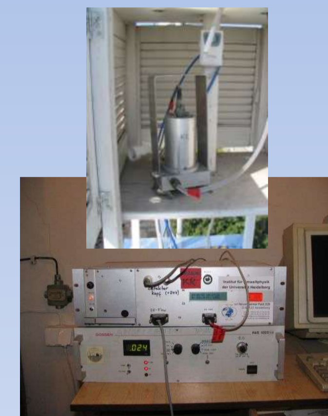
Fig 5. Radon monitor. Upper picture – measurement head, lower picture – electronic module
