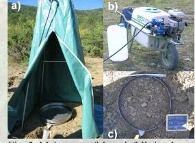
Fig. 2: Main parts of the rainfall simulator.
