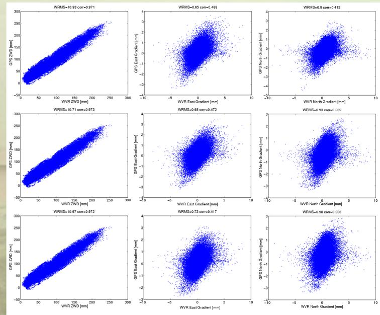
Fig 3: Scatter diagrams for the ZWD, the east, and the north gradients estimated from the WVR and the GPS observations. The GPS estimates use three different elevation cutoff angles: 5° (top), 10° (middle), and 15° (bottom).
