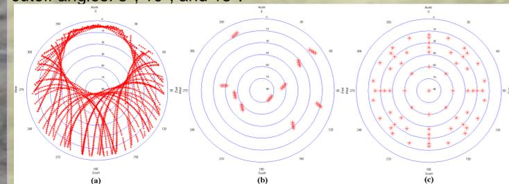
Fig 1: The sky distribution of observations by the ONSA GPS receiver during October 23, 2007 (a) for the whole day, and (b) for 15 minutes starting at 0:00 UTC, and (c) one cycle of 63 WVR observations, which takes about 15 min.
