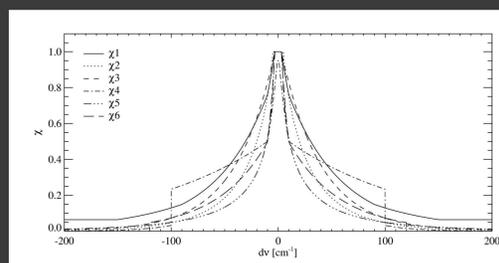
Figure 3. Line shape factors from each references (x1[8], x2[7], x3[9], x4[10], x5[12] and x6[11]).
