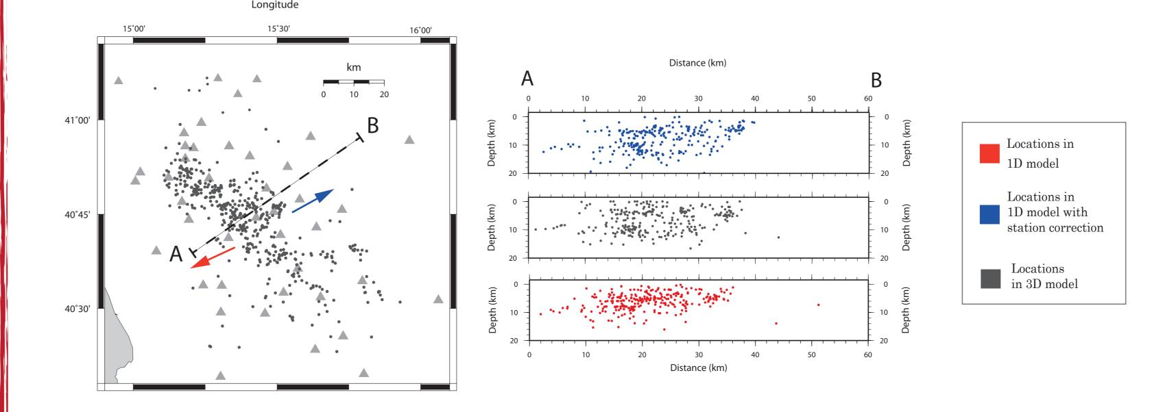
Analyzing the difference between the observed and computed travel times for the different velocity models we generally observed a better distribution of P-residuals respect to the S-residuals. Moreover there is a **gradual improvement in terms of RMS** when we considered the location in 1D model, the
