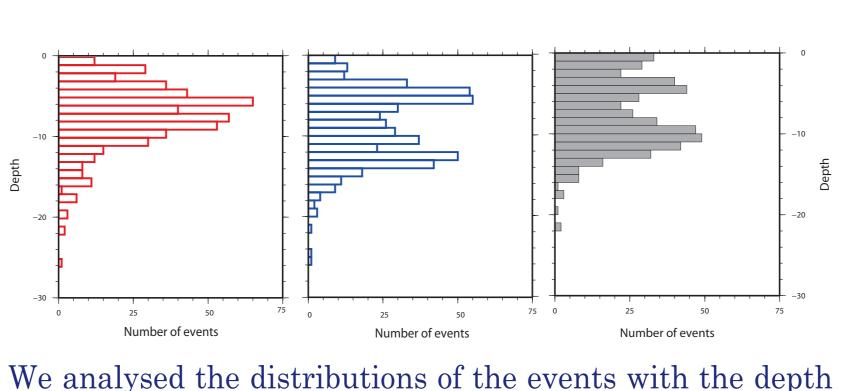
for the three velocity models. The seismicity appears more concentrated in the first 10 km depth in the 1D velocity
