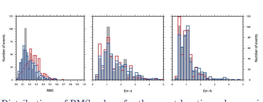
Distributions of RMS values for the event locations show a significant variation for 1D locations (average RMS=0.25 s), 1D locations with static corrections (RMS=0.19 s) and 3D locations (RMS=0.17 s).
