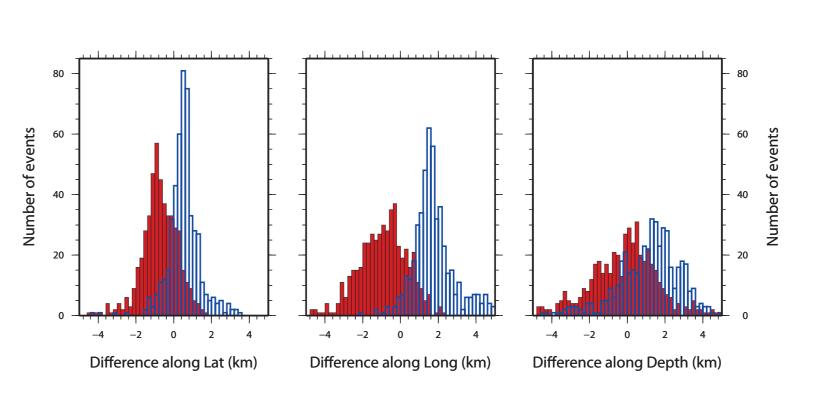
The histograms of the differences between the 1D and 3D locations along latitude, longitude and depth quantifies the shift respect to the 3D location (red: 1D model; blue: 1D model considering the station corrections). It appears to be more important along the Longitude.
