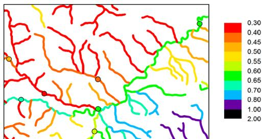
Figure 2. Example of estimation of streamflow (normalised specific 100-year flood [m<sup>3</sup>/s/km<sup>2</sup>], Mur region) along the river network with TOPKRIGING technique (Skøien et al., 2006)
