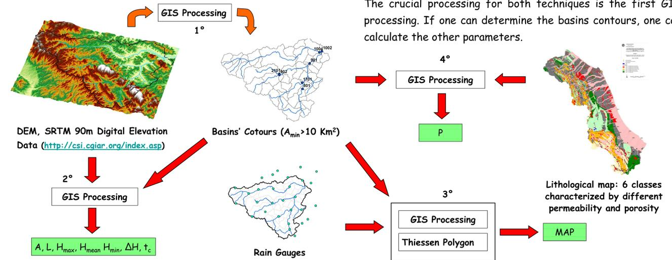
The crucial processing for both techniques is the first GIS processing. If one can determine the basins contours, one can calculate the other parameters.
