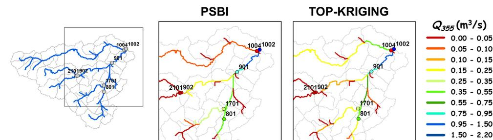
Figure 7 and 8. Comparison of techniques for estimating  $Q_{355}$  along the river network: the observed values are represented as colored dots, the estimated values are represented as colored lines.
