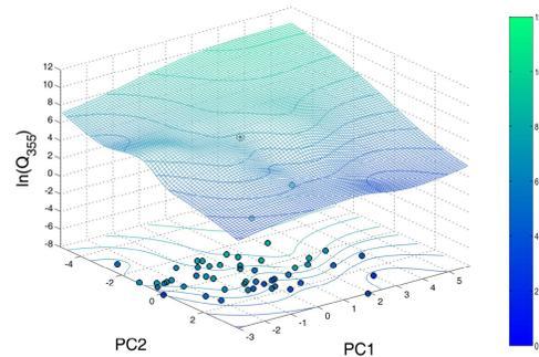
Figure 3. Example of cross-validation of PSBI: 3D representation of the surfaces generated in the physiographic space by the interpolation techniques (cross-validation site: River Aterno at L'Aquila).
