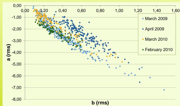
Parameters  $a$  (rms) and  $b$  (rms) of all plate measurements. The surface turns rougher as the melting season starts in April 2009. March 2010 matches March 2009 well even though the snow pack development conditions have been different in 2009 and 2010. March 2010 was warmer than March 2009 but the melting period had not yet started.
