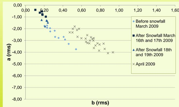
Parameters  $a$  (rms) and  $b$  (rms) of Tähtelä measurements from 2009. The effect of a snow fall event the 16th March 2009 has a clear effect on the snow surface roughness. During April 2009 there were no big snow fall events during the measurement period.
