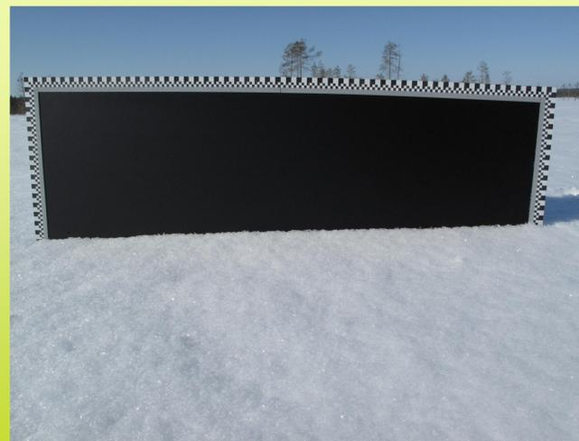
1. A black board with scales on the sides is partly inserted into the snow and a photo is taken of the plate and the snow-plate interface
