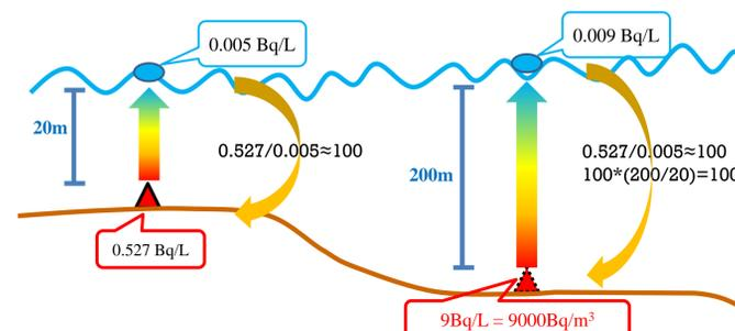
Fig. 6 A simple calculation of radon activity for the deeper hydrothermal vent.
