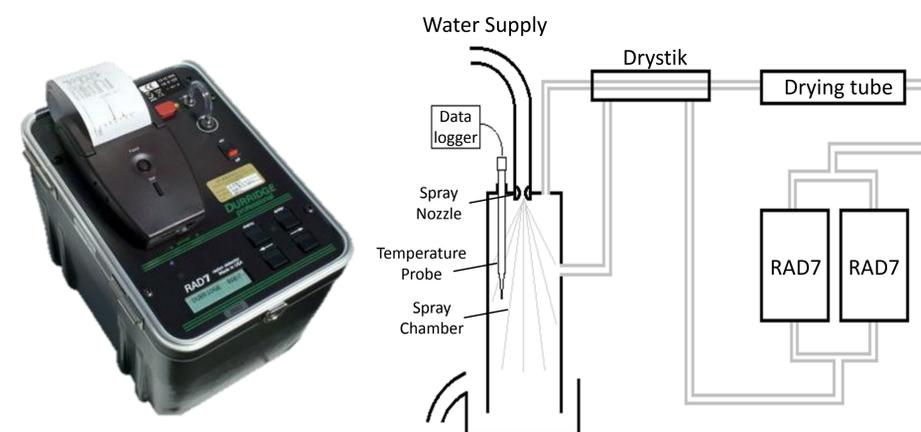
Fig. 2 RAD7 and Schematic diagram of the multi-RAD-AQUA system.
