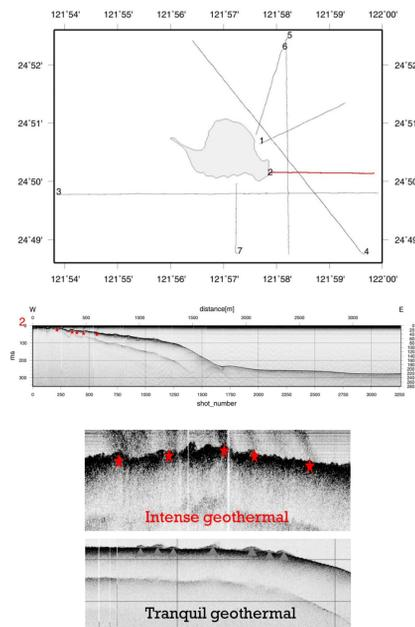
Fig. 3 Chirp sonar profile of track line 2 and two morphologies of hydrothermal vents.
