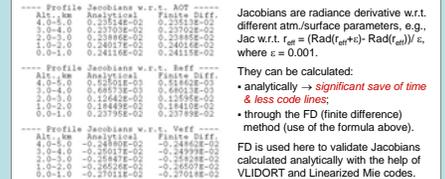
Jacobians are radiance derivative w.r.t. different AT surface parameters, e.g., Jac w.r.t.  $r_{eff} = (Rad(r_{eff}+) - Rad(r_{eff}))/r_{eff}$ , where  $r_{eff} \leq 0.001$ .
