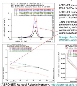
AERONET spectral channels: 340, 380, 440, 500, 675, 870, 1020 & 1640 nm.
