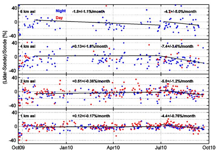
Fig. 3: Temporal evolution of the water vapor mixing ratio differences between lidar and sonde at different altitude levels.
