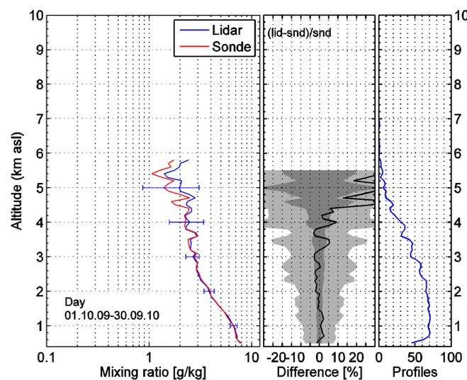
Fig. 4: Mean water vapor mixing ratio (left) and mean bias (middle) during day. Number of profiles (right).
