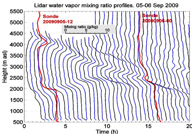
Fig. 2: Lidar water vapor mixing ratio time-series (blue and black) with radiosonde profiles (red).
