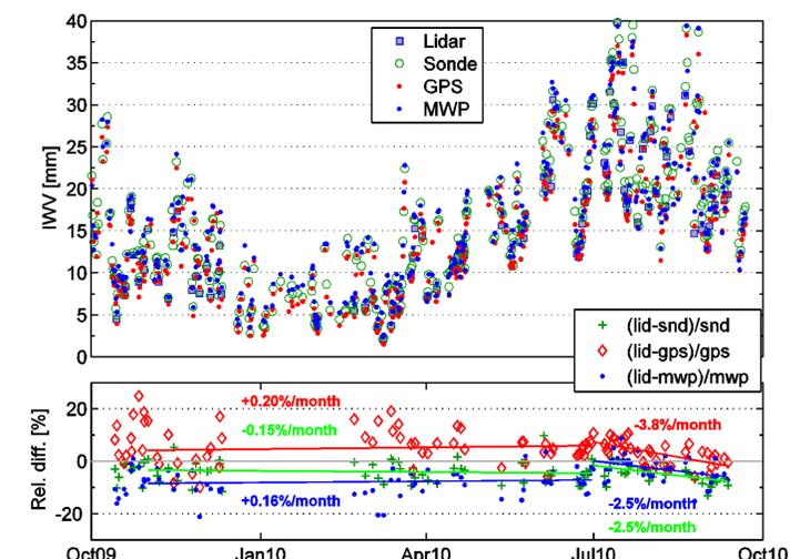
Fig. 6: Top panel: Integrated water vapor time-series above Payerne retrieved from lidar, radiosondes, GPS and microwave radiometer. Bottom panel: Relative difference.
