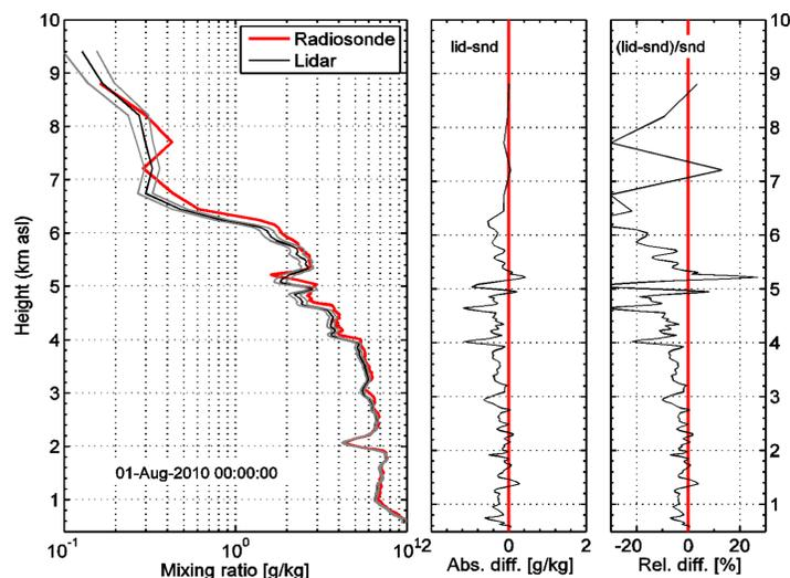
Fig. 1: Example of night-time water vapor mixing ratio profiles from lidar and radiosondes (left). Absolute and relative differences (middle and right).
