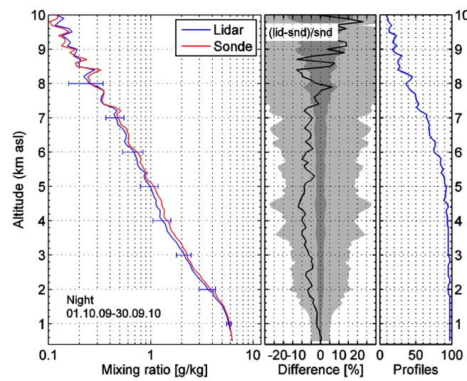
Fig. 5: Mean water vapor mixing ratio (left) and mean bias (middle) during night. Number of profiles (right).
