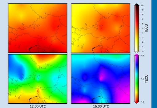
Fig. 4 Difference between CODE TEC map and maps generated with the kriging method (top) and difference between CODE RMS and kriging standard deviation (bottom)
