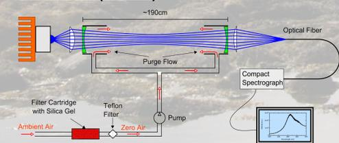
Figure 4: CE-DOAS basic set-up principle.
