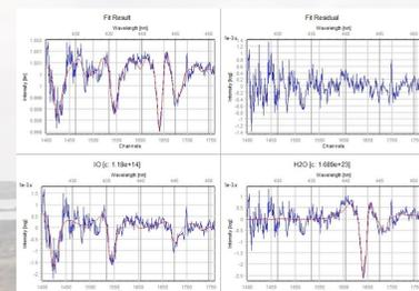
Figure 3: LP-DOAS IO evaluation. Spectrum from 02/06/2011 12:01 UTC measured at MRI over 1890m (Retro 3). IO concentration  $12.4 \pm 2.2$  ppt.
