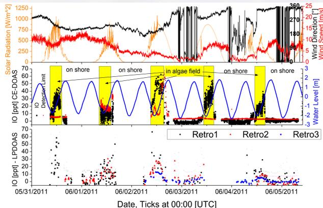
Figure 7: Meteorological data and IO values from MRI. During low tide very high IO concentrations of up to ~60ppt are observed in the algae field with both instruments. Note that the short LP-DOAS light path (Retro1) has a larger detection limit and measurement error (not drawn for simplicity)
