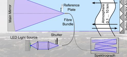
Figure 2: LP-DOAS basic set-up principle.
