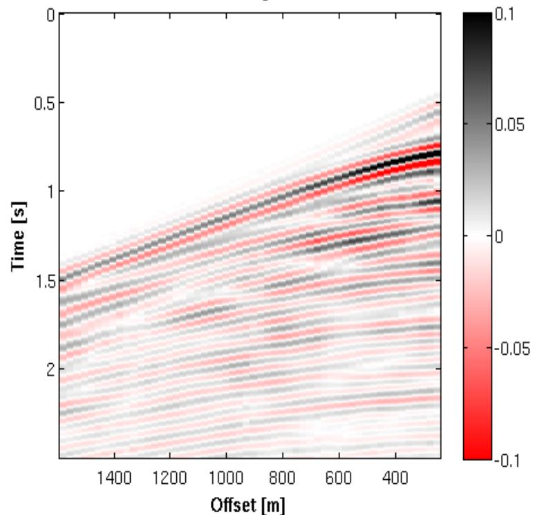
Data pre-processing: Noise attenuation, spreading transformation, near offsets
