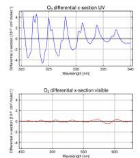
Figure 2: Direct comparison of the differential ozone absorption cross-sections in the Huggins bands (top) and the Chappuis band (bottom)
