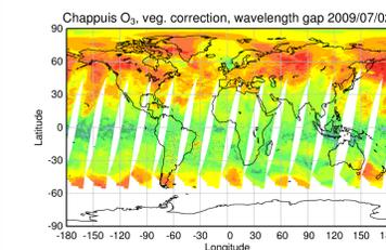
Figure 4: One day of ozone columns retrieved in the Chappuis band without vegetation correction (top), with correction (middle) and with correction and excluding values from 500 - 515 nm (bottom).
