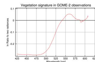
Figure 5: Logarithm of the ratio of two measurements, one having a large residual over vegetation and one close by producing a good fit. This ratio has been included in the fit to correct for vegetation effects.
