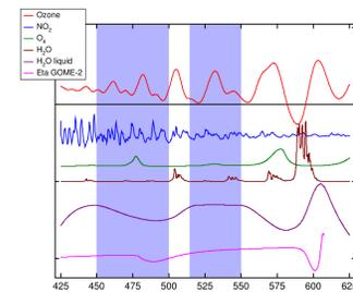
Figure 3: Relevant absorption cross-sections in the Chappuis band. Values are shown in arbitrary units and have been high pass filtered (O<sub>3</sub>, NO<sub>2</sub>, H<sub>2</sub>O<sub>liquid</sub>). The shaded area is the fitting window used.
