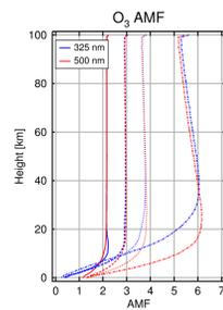
Figure 1: Block air mass factors (weighting functions) for the Huggins and Chappuis bands. Values for SZAs 30°, 50°, 60°, and 80° are shown from left to right. Surface albedo was set to 0.05.
