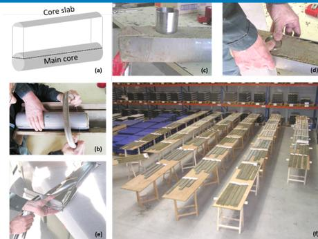
**Figure 1:** Core sampling at SCK·CEN: a) schematic of slab removal from main core, b) incision is made in main core to the appropriate depth for slab removal, c) 100 cm<sup>3</sup> steel core for hydraulic conductivity determination in the lab, d) steel core inserted in core material, e) vacuum sealing of main core for long-term storage, f) display of core slabs for geological description.
