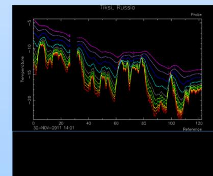
Time series of the soil temperature at different levels for the Tiksi site obtained during December 2011-March 2012. Note a remarkable a warm event in February 2012, lasting about two weeks, has impacted soil temperature dramatically. The big warm-up event was due to the coupling of the Aleutian Low and high pressure ridge extending well into the Arctic western Canada.
