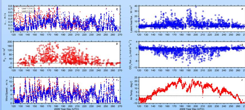
Time series of the hourly averaged (a) friction velocity, (b) sensible heat flux ( $H_s$ ), and (c) wind speed for the Eureka site obtained during May-September 2009 (YD 120-270). Measurements were made by sonic anemometers located at 3 and 8 m above the surface. Positive values of  $H_s$  correspond to the unstable (convective) conditions and vice versa. Hourly averages of the sensible heat flux show large diurnal variations during summer.
