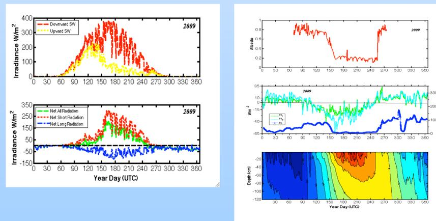
Annual cycles of the daily averaged short-wave radiation (Kipp&Zonen CM22) and the net radiative energy, measured at the Eureka Flux Tower during 2009. Long-wave radiation component was measured by Eppley PIR
