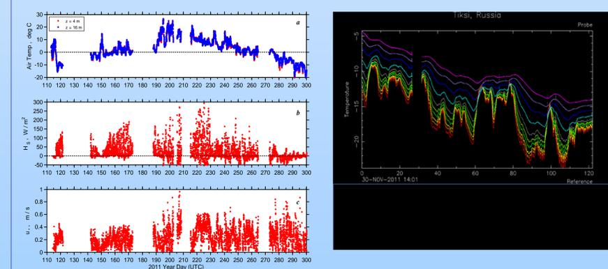
Time series of the 30-min averaged (a) air temperature, (b) sensible heat flux ( $H_s$ ), and (c) friction velocity for the Tiksi site obtained during April-October 2011 (YD 110-300). Measurements were made at 4 and 16 m above the surface. Positive values of  $H_s$  correspond to the unstable (convective) conditions and vice versa. Turbulent fluxes are based on the gradient method.
