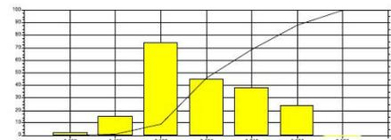
Fig. 2: Sieve analysis of soil used for the tracer tests.
