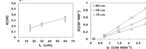
Fig. 8: Trend of  $\alpha_L$  vs scale (continuous inlet). Fig. 9: Trend of  $D_L$  vs velocity (continuous inlet).
