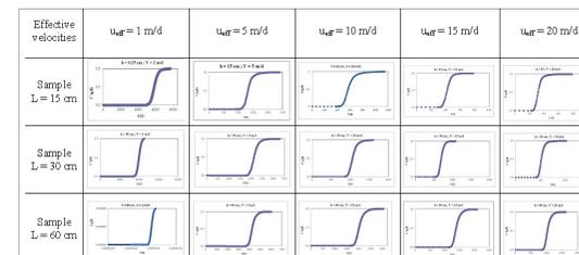
Fig. 5: Breakthrough curves for continuous inlet.
