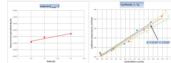
Fig. 6: Trend of  $\alpha_L$  vs scale (inlet in short time). Fig. 7: Trend of  $D_L$  vs velocity (inlet in short time).
