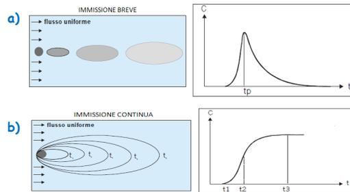
Fig. 1: Conceptual model of mass propagation for a) in short time and b) continuous inlet.
