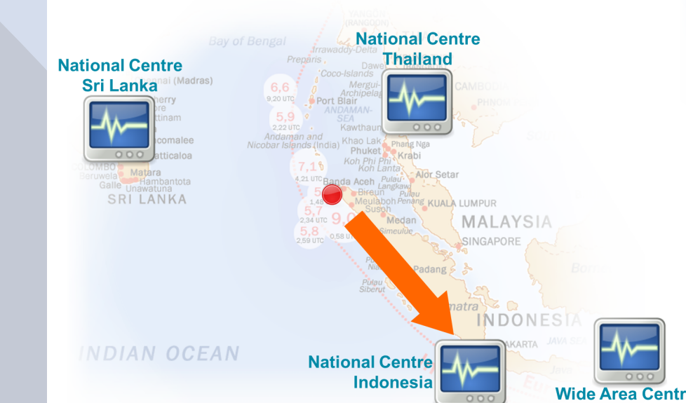
Fig. 6d. Indonesian disseminates local/national tsunami warnings based on sensor measurements and tsunami simulations/forecasts.
