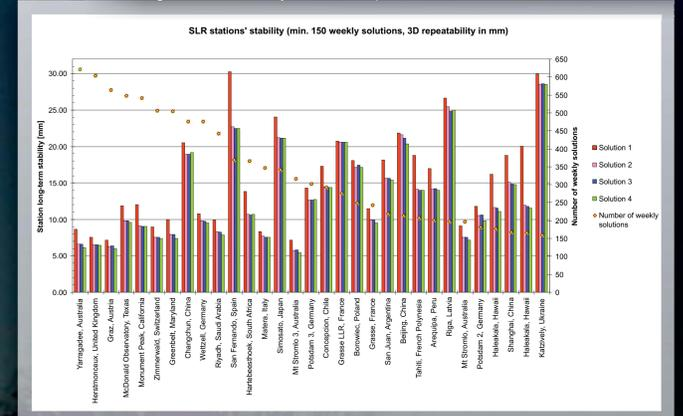
Fig. 10. The 3D stability of SLR stations for Solution 1, Solution 2, Solution 3 and Solution 4. The improvement of SLR stations repeatability due to ANTL (3.5%) is smaller than for GNSS stations (20%), because the GNSS network contains well-performing in-land stations. In the SLR network the station distribution is uneven with no well-performing in-land sites.
