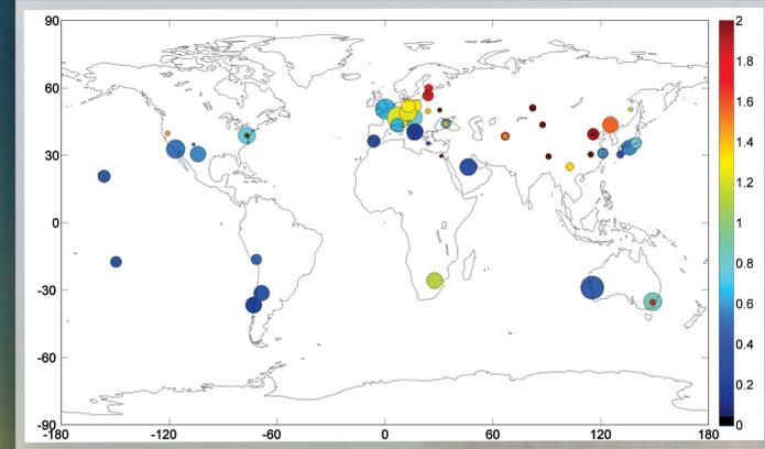
Fig. 7. Assessment of the impact of Blue-Sky effect on SLR stations using mean APL vertical correction applied on SLR stations (the size of circles denotes number of weekly solutions). The Blue-Sky effect (the difference between vertical displacement correction, when SLR station observes and the mean displacement, which supposes to be zero) is more than 2 mm for in-land stations.
