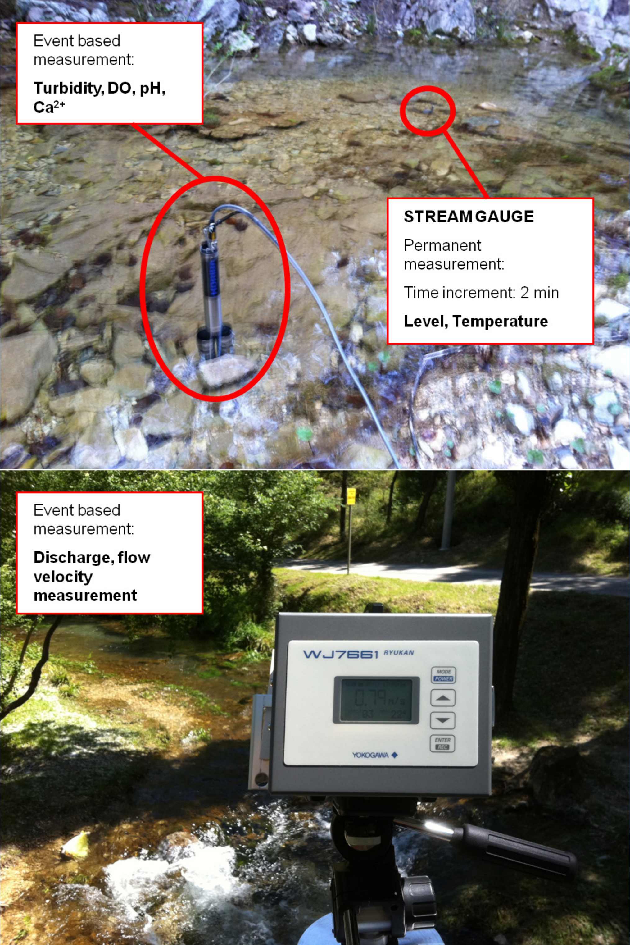
Event based measurements on the stream and permanent measurement of water level and water temperature on five locations.
