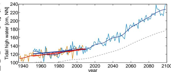
**Figure 2:** Possible rise of the mTHW<sub>1</sub> (simulated light blue, measured orange), mTHW<sub>10</sub> (simulated dark blue, measured red), and trend (simulated blue, measured red), mean sea level (MSL, NN + 100cm, dashed grey).
