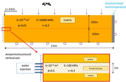
Fig. 1 – Model geometry and boundary conditions.
