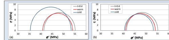
Fig. 5 – Stress state at the contact with the matrix (a) and inside the fractured zone (b) at 3 m away from the injection well. After 10 days of cold water injection, stability is significantly reduced at the fracture-matrix contact, while inside the fracture it is comparable to that of the isothermal case.
