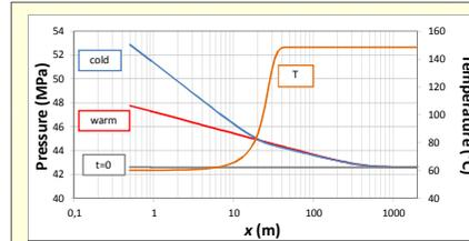
Fig. 2 – liquid pressure and temperature vs distance from injection well in the fracture filling after 10 days of warm/cold water injection. Overpressure results greater when accounting for cold water because the temperature drop reduces the hydraulic conductivity. Note the change in the slope of the overpressure coinciding with the cooling front in the cold water injection simulation. Note also the difference in hydraulic and thermal response time.
