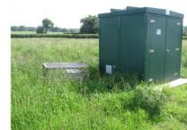
ISCO automatic samplers in bankside monitoring stations are remotely triggered to capture 1 litre stream water samples every 60-120 minutes during a storm, capturing the entire event in high-resolution.
