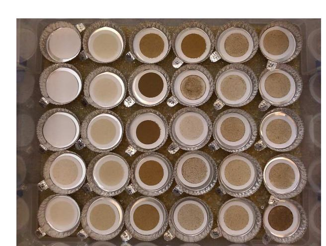
All water samples are vacuum filtered through quartz fibre filter (QFF) papers to extract the suspended solids. Source area sediments are also transferred onto QFF papers after being wet sieved to 63 µm to extract the fine silts and clays that become suspended in-stream. These filter papers are subsequently analysed by both XRF and DRIFTS to determine the concentrations of major elements and compounds.
