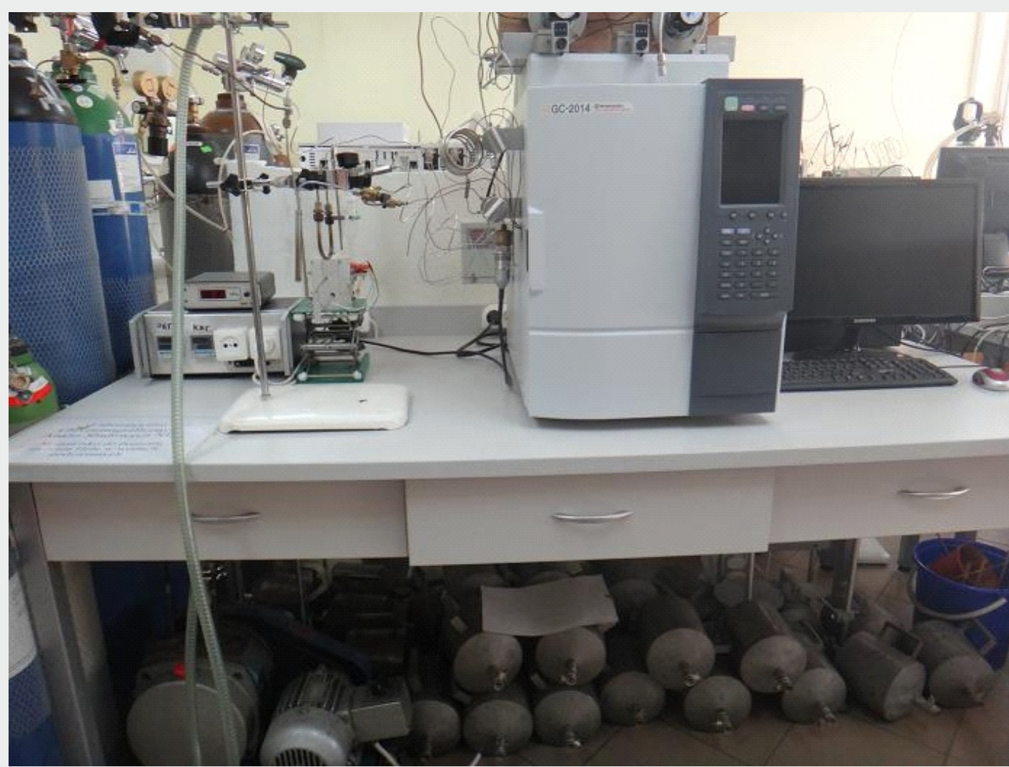
Figure 5. Scheme and the picture of the system for helium concentration measurements.
