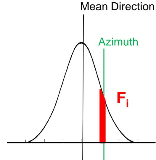
Valid energy flux for a sea state  $i$  ( $F_i$ ) depends on the difference between the mean wave direction and the azimuth.
