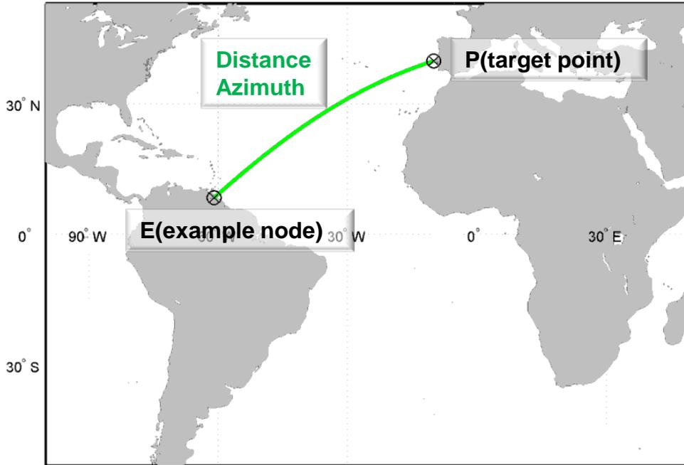
The azimuth is the angle formed between North and a line from the example node to the target point
