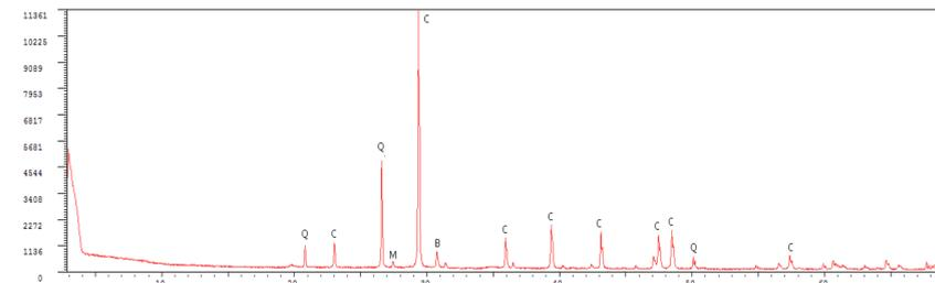
Figure 2. X-Ray diffraction (XRD) analysis of unburnt soil sample. Identification of different mineral in the sample. Q (Quartz), C (Calcite), M (Microcline) and B (Blixite)
