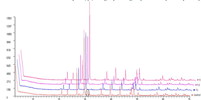
Figure 3. X-Ray diffraction analysis of soil samples heated at 300 (F1), 500 (F2) and 700 °C (F3), and unheated soil samples (control). The peak associated to blixite is marked.
