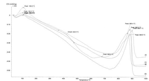
Figure 5. Differential thermal analysis of unburnt soil sample and unburnt soil samples exposed to different temperatures. Unburnt soil sample Line [1], unburnt soil sample exposed to 300°C Line [2], 500°C Line [3] and 700°C Line [4].
