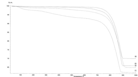
Figure 4. Thermogravimetric analysis of unburnt soil sample and unburnt soil samples exposed to different temperatures. Unburnt soil sample Line [1], unburnt soil sample exposed to 300°C Line [2], 500°C Line [3] and 700°C Line [4].
